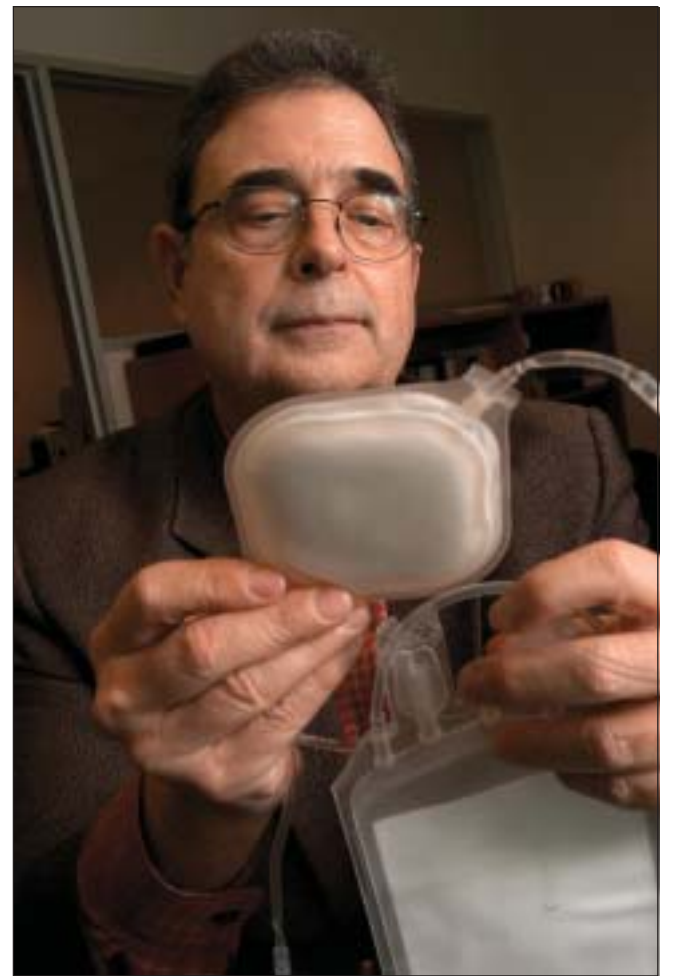
Dr. Ruben Carbonell examines a filter filled with resin beads that were effective in removing harmful prion proteins from the blood of infected animals. The finding has major implications for the removal of prion proteins during blood transfusions. (Photo by Roger Winstead)
