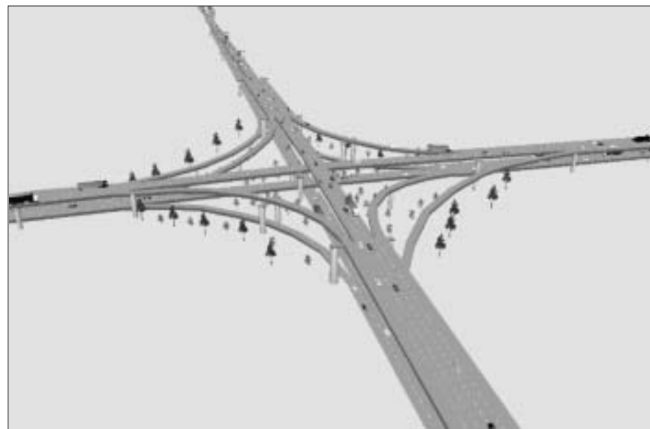
The nano-interchange relies on all-directional connections, combinations of left- and right-hand entrances and exits and four levels of freeway and ramp structures to minimize right-of-way. (Image courtesy of Meredith L. Harris).
