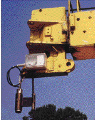
A Black Box Technology sensor on the tip of a crane senses whether or not the hoist line is in a nonvertical position.
