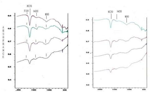
**Fig. 3a.** FTIR of KBr pellets of 5 min oxidized aspen charcoal – samples A,B and C and KBr (top).
