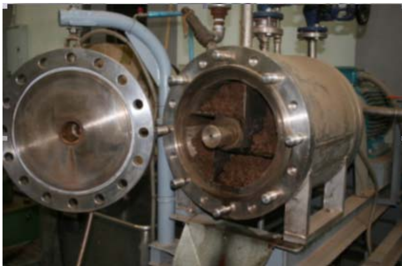
Fig. 2. Laboratory autoclave used for the thermal treatment of the rubberwood fibers
