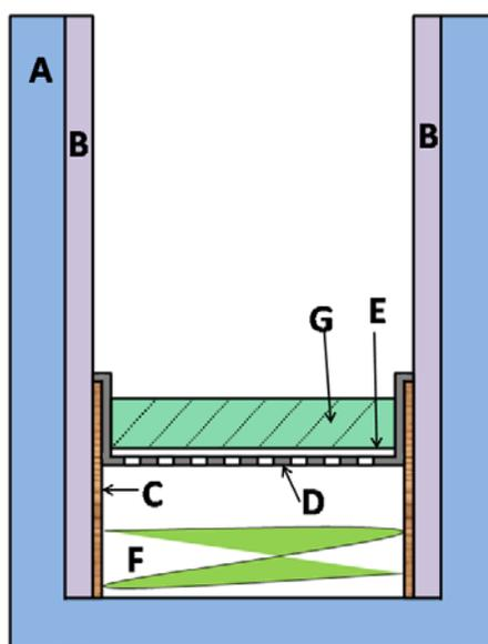
**Fig. 2.** Scheme of water retention value measurement setup for centrifuge, A: Centrifuge bucket, B: Adapter, C: Spacer, D: Stainless steel cap with holes, E: Filter paper/Membrane, F: Tissue for water absorption, G: Sample
