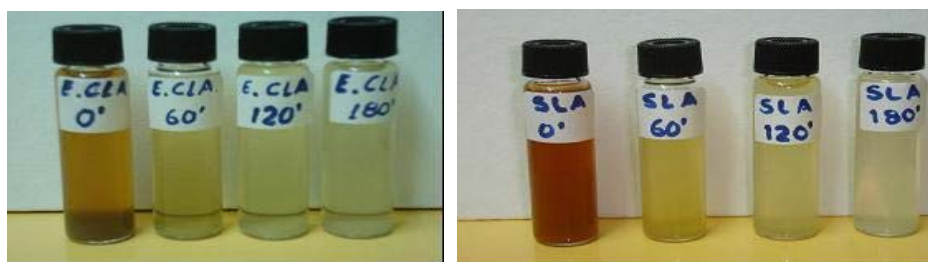
Figure 5. Ozonation of centrifuged samples of diluted liquor and of effluents from the aerated lagoon
