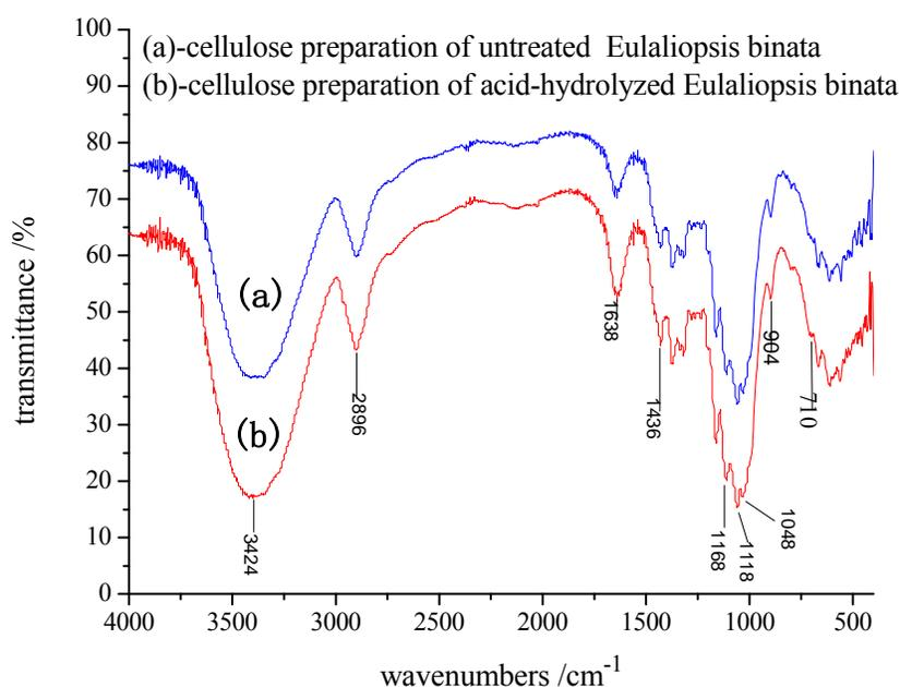
**Fig. 2.** FTIR spectra of cellulose preparations
