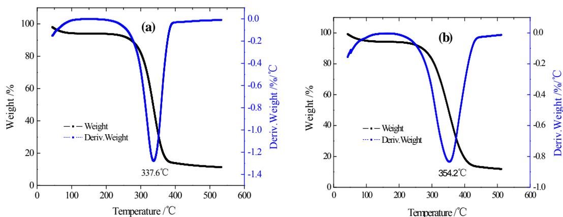
**Fig. 5.** Thermal properties of the cellulose preparations of untreated (a) and acid hydrolyzed (b) *Eulaliopsis binata*
