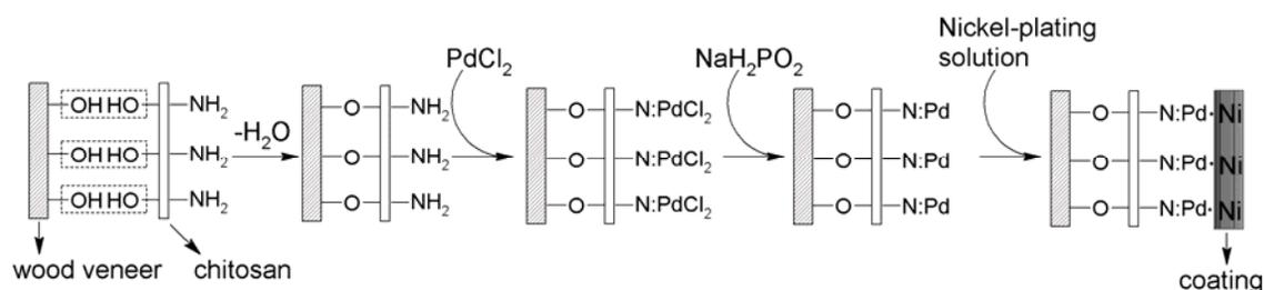
**Scheme 3.** Proposed mechanism of the activation and plating process
