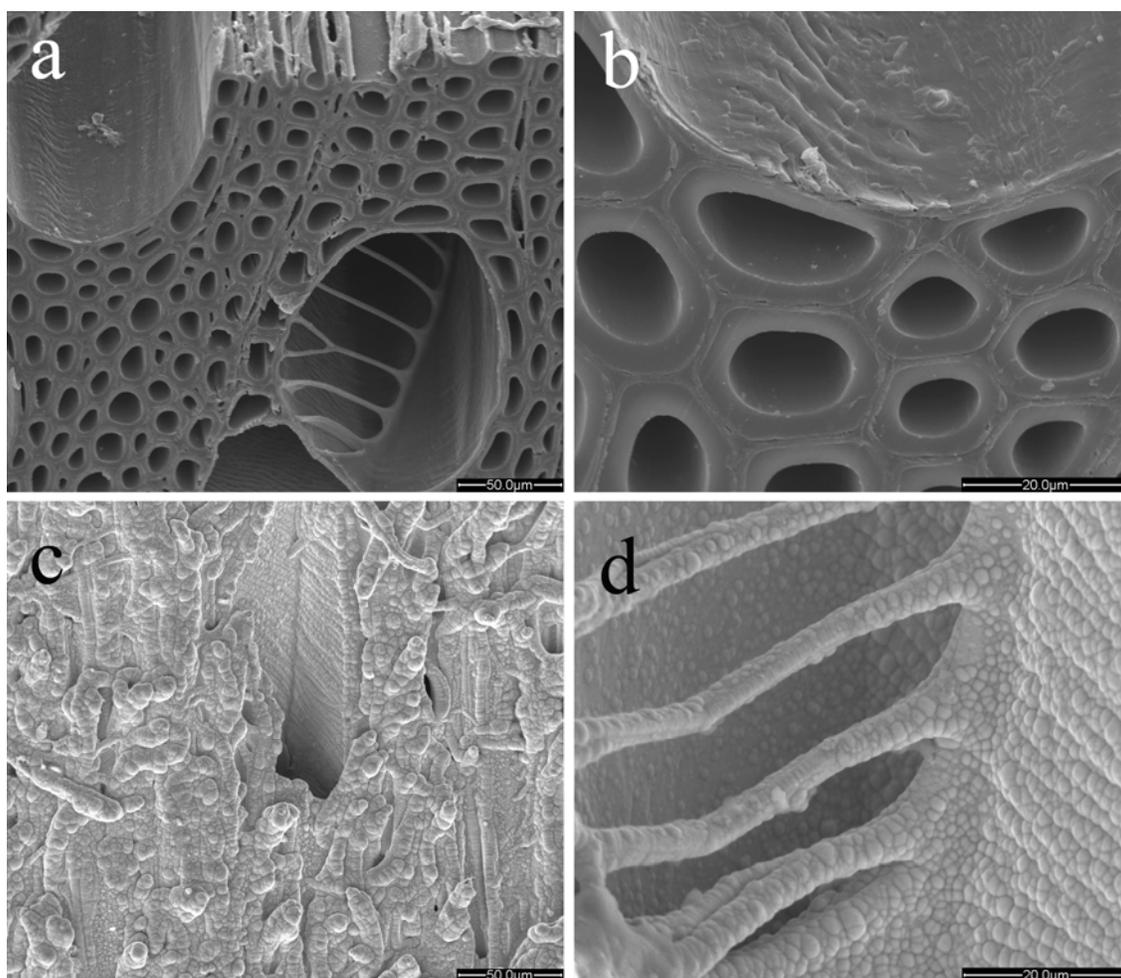
**Figure 2.** SEM photographs of the raw (a×500, b×1000) and plated wood veneers (c×500, d×1000)
