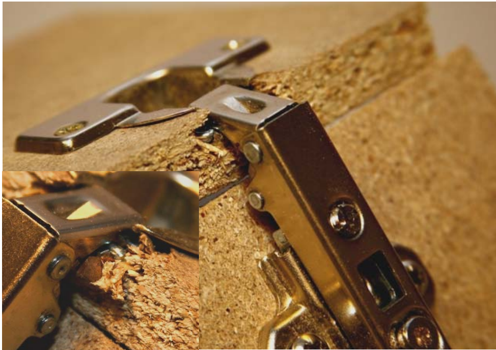
Fig. 17. Example of testing of hinge bearing connection
