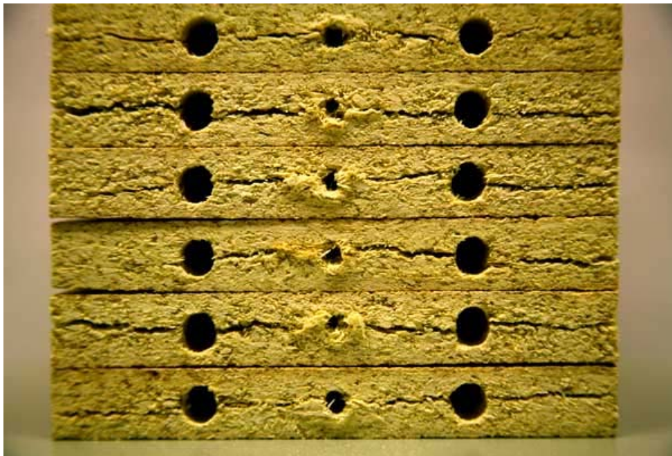
Fig. 15. The delamination of the panels r600 from connections with confirmat
