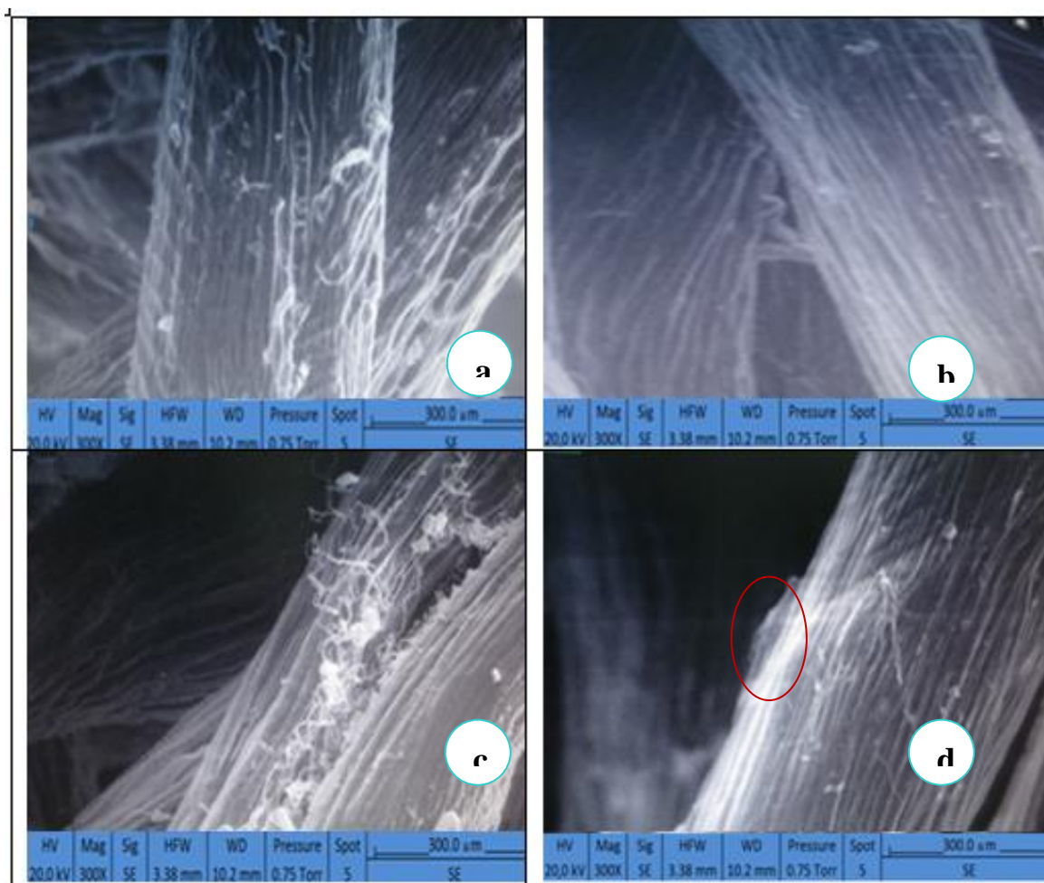
Fig. 1. SEM photos of untreated and treated luffa fibers: a) untreated, b) alkali treated, c) treated with combined process, d) acetylated
