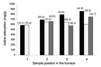
**Figure 3.** lodine adsorption and yield of AC from wood charcoal. , first trial for AC production; , second trial; , third trial. The value in parenthesis is yield. The number of sample position means the basket position from the bottom of furnace.
