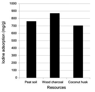
Figure 4. lodine adsorption of AC from different raw materials.
