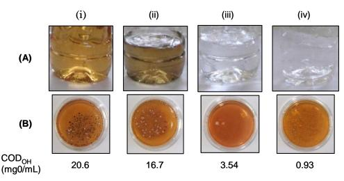
**Figure 5.** Decoloration (A) and bacterial colonization of the creek water in University of Palangka Raya purified by type B apparatus. See detail of this apparatus in Figure 2. (i), after purification with keranggas; (ii), with keranggas followed by charcoal; (iii), with charcoal followed by AC with 870 mg/g of iodine adsorption; (iv), with AC followed by keranggas. The initial COD<sub>OH</sub> of this creek water was 20.0 mgO/mL.
