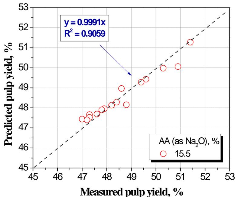
**Fig. 5.** Comparison the experimentally measured and predicted pulp yields of fast-growing *Eucalyptus* with the AA charge of 15.5%
