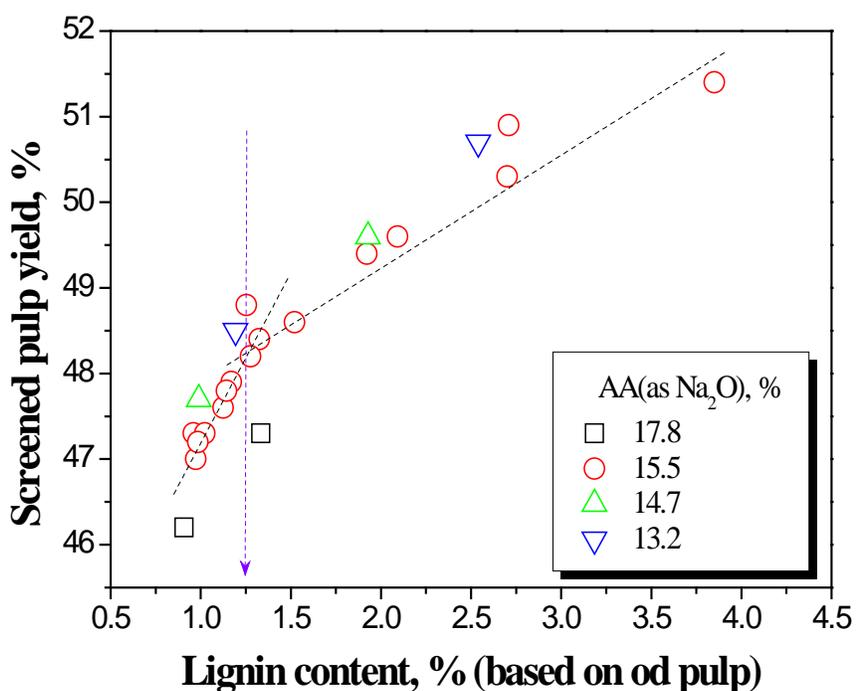
Moreover, the ability to fit the data to two straight lines based on results from an AA change of 15.5% indicated that a transition existed from bulk to residual phase of delignification. Initially, pulp yields decreased slowly with the change of lignin content. Then, pulp yields decreased faster than they did in the first stage, which could be revealed by the slopes of two linear fitting functions in Fig. 1.
