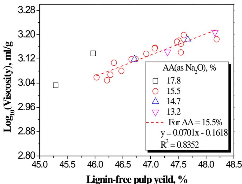
Fig. 3. The change of lignin-free pulp yields with the logarithm of pulps viscosities
