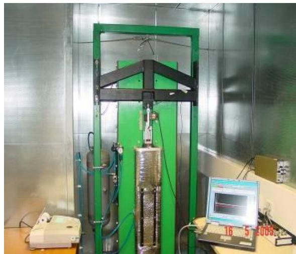
**Fig. 1.** Impact test rig for measuring the strength properties of wet papers. The output consists of tensile strength, strain at break, dynamic tensile stiffness, and residual tension
