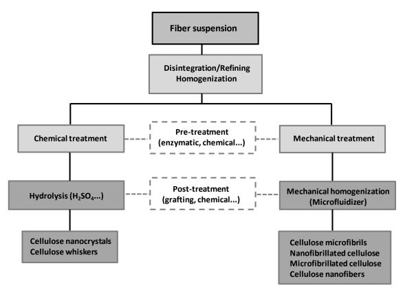
Fig. 1. Schematic overview of approaches to produce nanocellulosic materials from fibers.
