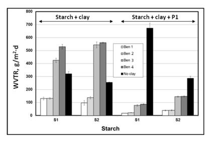
**Fig. 5.** WVTR values obtained at 23°C and 50% RH for selected combinations of starch, plasticizer and clay coated on low basis weight paper at a coat weight of 15-20 g/m<sup>2</sup>
