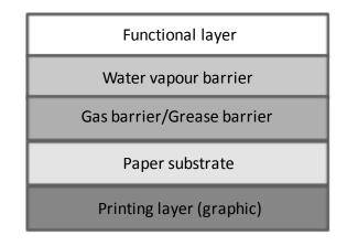
Fig. 7. Typical multilayer coating structure.
