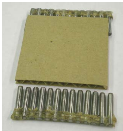
Figure 10. Photograph of the dowel pin assemblies used to for crushed boards and T 839
