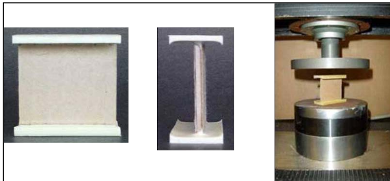
Figure 3. An ECT sample embedded in supporting epoxy resin strips front and side views and (right) mounted between the platens of a compression tester
