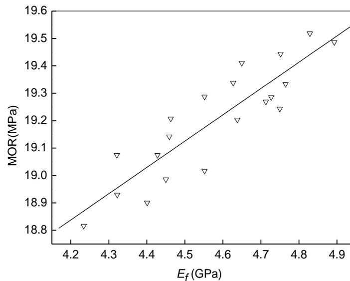
**Fig. 3.** Regression curve between  $E_f$  and MOR of wood-plastic planks of Group 1
