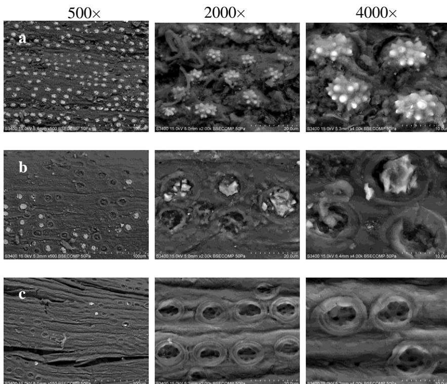
**Fig. 1.** SEM images of (a) untreated OPEFB, (b) OPEFB treated by autoclaving at 121 °C for 5 minutes, and (c) OPEFB treated with 0.5% NaOH followed by autoclaving at 121 °C for 5 minutes
