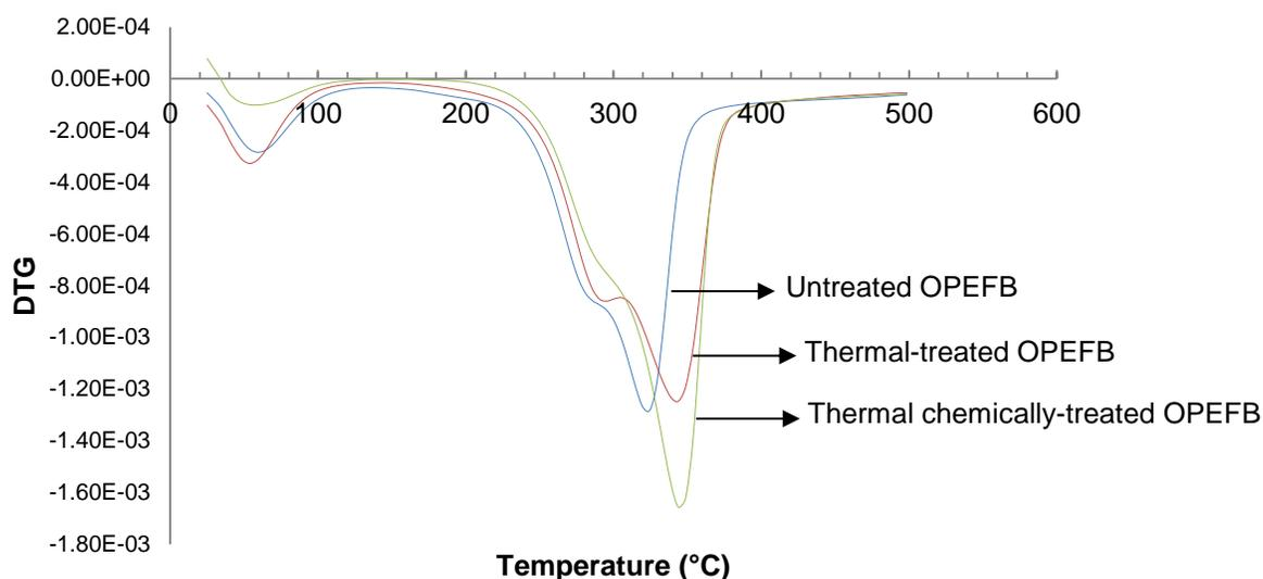
Fig. 4. TG (a) and DTG (b) curve of untreated and treated OPEFB samples
