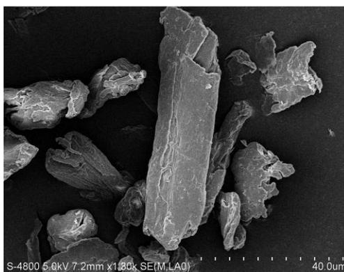
Fig. 1. FE-SEM micrograph of MCC
