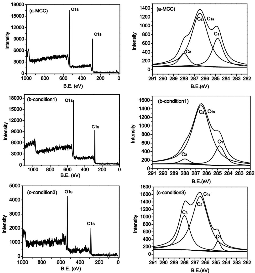
**Fig. 4.** C(1s) and O(1s) XPS survey spectra of (a) MCC, (b) CNWs from condition 1, and (c) CNWs from condition 3
