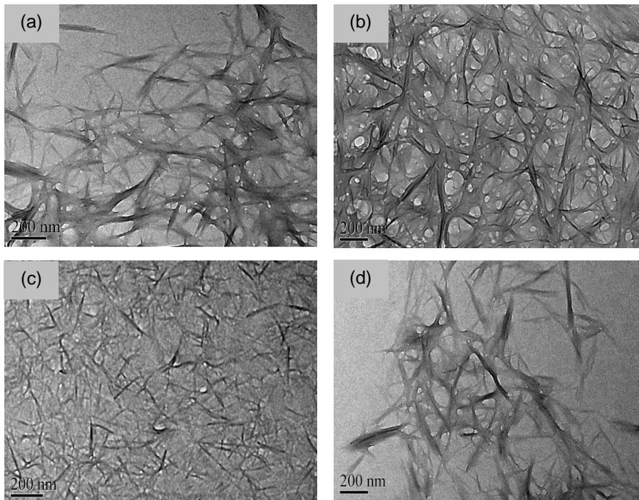
**Fig. 2.** TEM micrograph of CNWs with treatments (a) condition 1, (b) condition 2, (c) condition 3, and (d) condition 5
