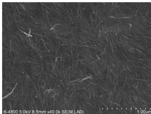
**Fig. 3.** FE-SEM micrograph of CNWs treated with condition 3
