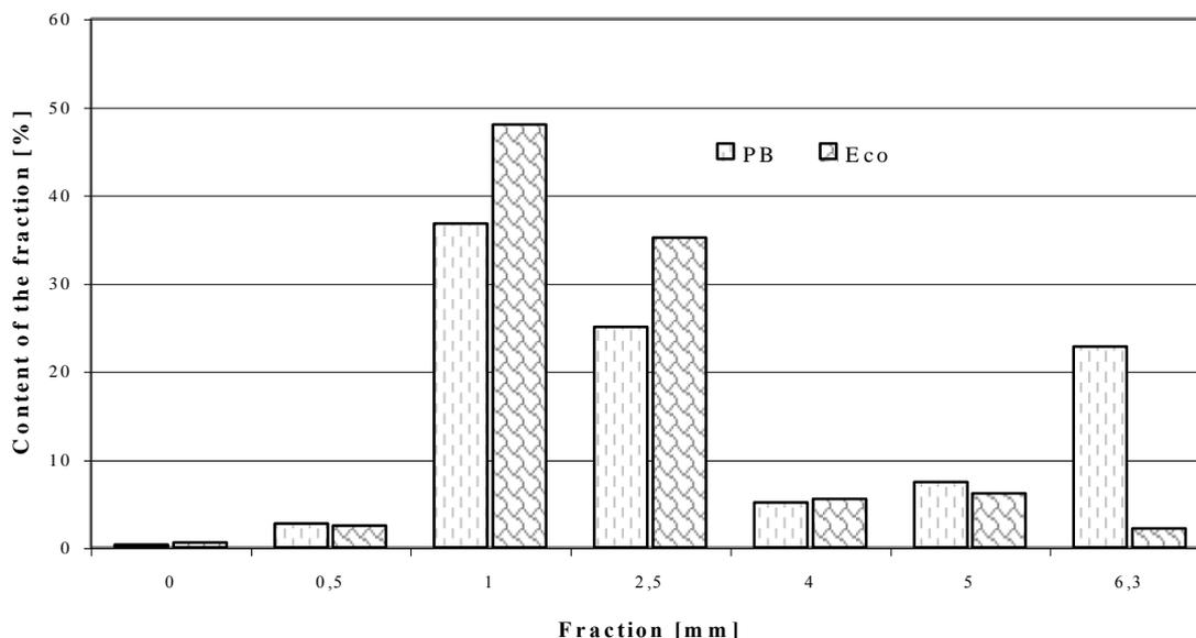
**Fig. 1.** Fractional composition of small chips (PB – chips intended for the core layer of particleboards, Eco – chips produced by comminution of unrefined particleboards)
