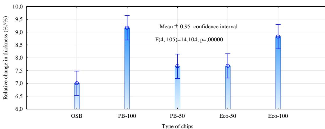
**Fig. 6.** Relative change in thickness of laboratory OSB determined over the entire seasoning process
