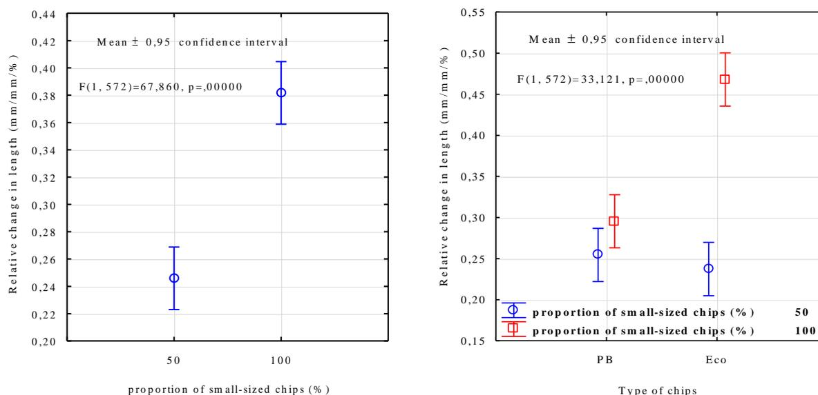
**Fig. 3.** Effect of the type of chips in the OSB core layer on the changes in length observed for various humidity conditions (analysis only for Eco PB chips); a) effect of fine chips share, and b) relationship between the chips type and share
