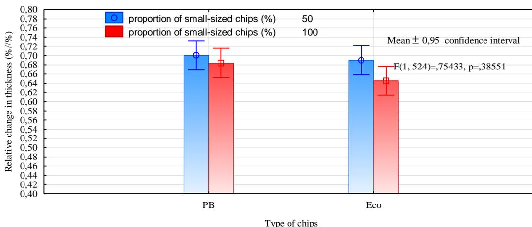
**Fig. 5.** Effect of type and share of fine chips in the core layer of OSB on the relative change of the board thickness, recalculated for 1% change in the board moisture content
