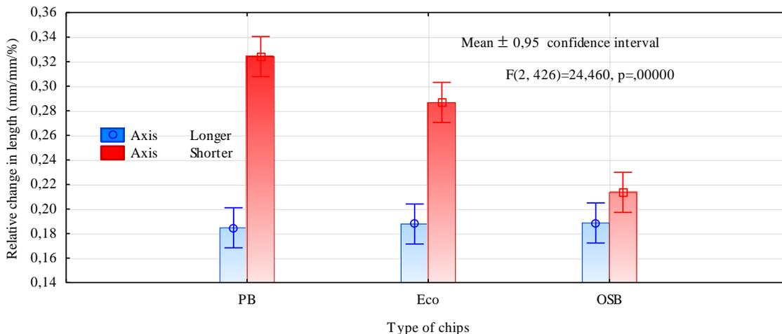
**Fig. 4.** Effect of the type of axis on the change in length for the boards containing 50% of fine chips (PB and Eco) or only strand chips (OSB) in the core layer
