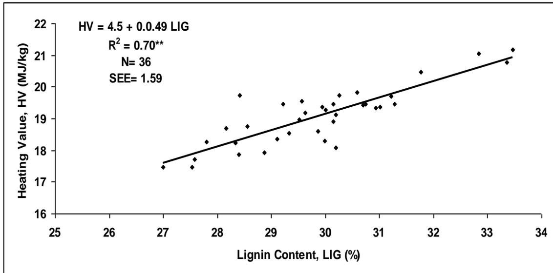
Fig. 5. Heating value of acacia wood versus lignin content
