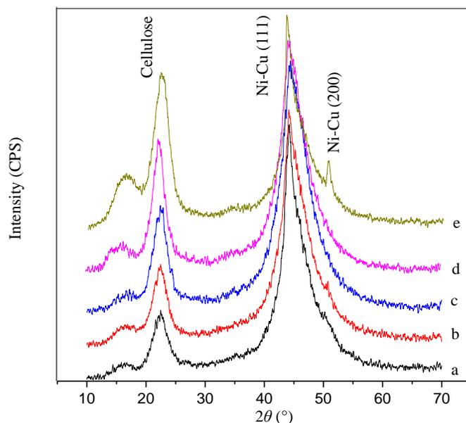
**Fig. 4.** XRD patterns of Ni-Cu-P-coated veneers with varying copper content: (a) 3.96 wt%, (b) 7.38 wt%, (c) 8.62 wt%, (d) 15.62 wt%, and (e) 20.73 wt%
