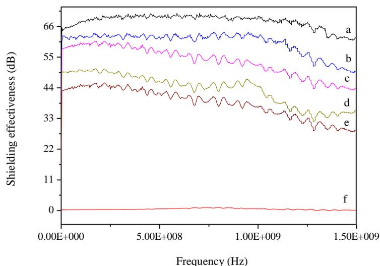
**Fig. 7.** Shielding effectiveness of Ni-Cu-P-coated veneers with different  $\text{CuSO}_4 \cdot 5\text{H}_2\text{O}$  concentrations: (a) 0.6 g/L, (b) 1.0 g/L, (c) 1.4 g/L, (d) 1.8 g/L, (e) 2.2 g/L, and (f) pristine veneer
