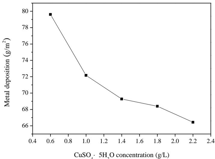
**Fig. 2.** Effect of CuSO<sub>4</sub>·5H<sub>2</sub>O concentration on metal deposition (pH 9.5, temperature 90 °C)
