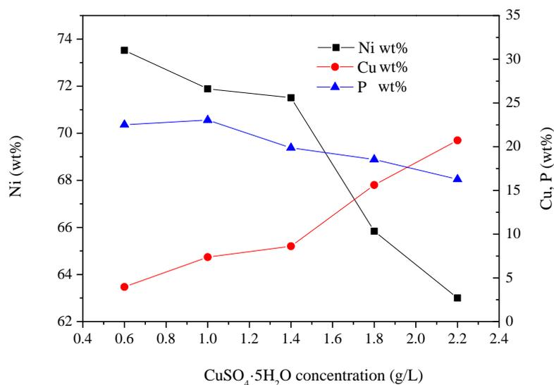
**Fig. 3.** Effect of  $\text{CuSO}_4 \cdot 5\text{H}_2\text{O}$  concentration on elemental composition of the coating (pH 9.5, temperature  $90^\circ\text{C}$ )
