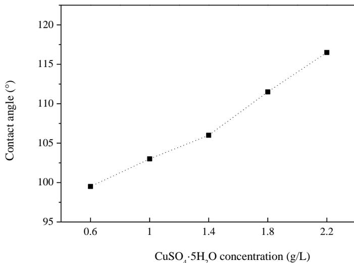
**Fig. 6.** Effect of  $\text{CuSO}_4 \cdot 5\text{H}_2\text{O}$  concentration on contact angle of the coating (pH 9.5, temperature  $90^\circ\text{C}$ )
