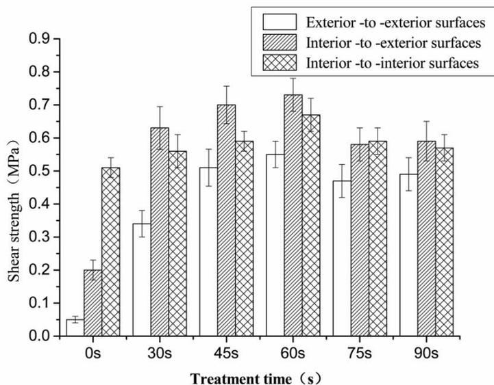
Fig. 8. Shear strength of the wheat straw
