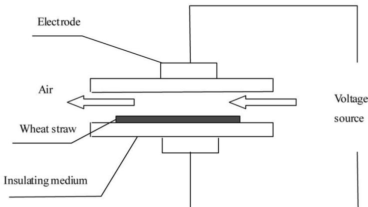
**Fig. 1.** Atmospheric pressure plasma processor
