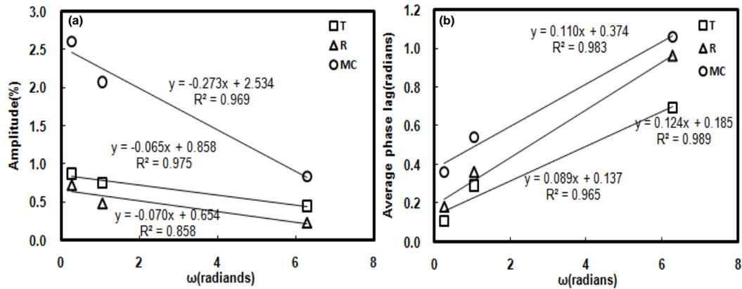
**Fig. 2.** Plots of amplitude (a) and phase lag (b) responses against angular frequency of RH cyclings (25 °C, 10 mm)
