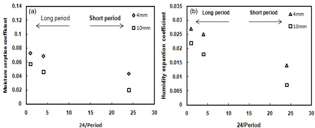
**Fig. 4.** Dynamic moisture sorption coefficient (a) and humidity expansion coefficient (b) at different cyclic periods for poplar wood (40 °C)
