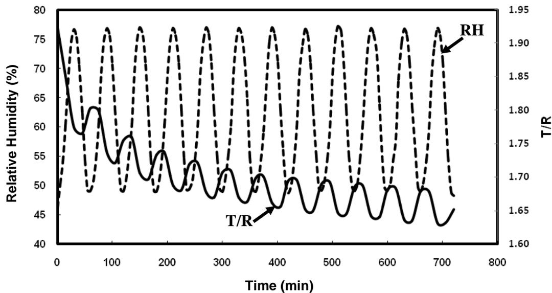
Fig. 6. Transverse anisotropy for 10-mm thick poplar wood cycled at 1 h (40 °C).
