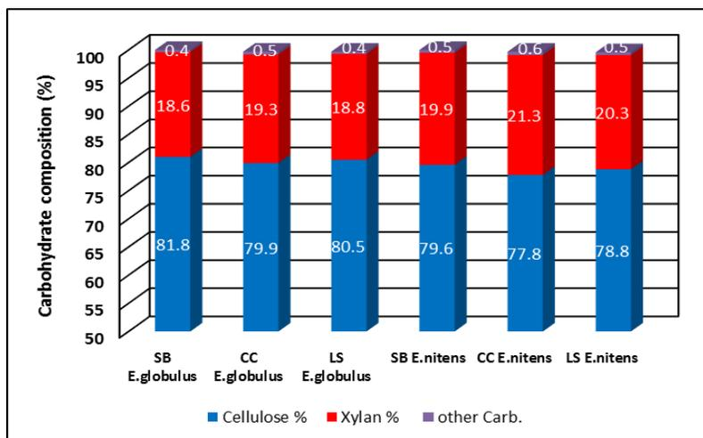
**Fig. 11.** Carbohydrate composition of fully-bleached pulps of *E. globulus* and *E. nitens*
