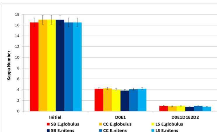
**Fig. 7.** Kappa numbers of *E. globulus* and *E. nitens* pulps during the  $D_0E_1D_1E_2D_2$  bleaching. The error bars present 95% confidence interval of the value.
