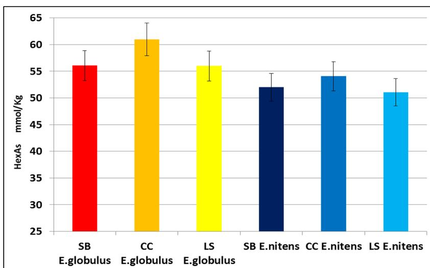
**Fig. 4.** HexA of brownstocks at kappa  $17 \pm 0.5$  for *E. globulus* and *E. nitens* for the three different cooking methods. The error bars present 95% confidence interval of the value.
