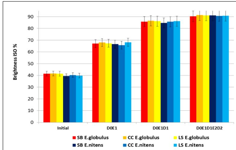
**Fig. 8.** ISO Brightness (%) development for *E. globulus* and *E. nitens* pulps during the  $D_0E_1D_1E_2D_2$ . The error bars present 95% confidence interval of the value.
