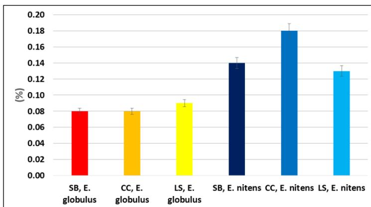
**Fig. 12.** Acetone extractives of fully-bleached pulps of *E. globulus* and *E. nitens* for the three different cooking methods. The error bars present 95% confidence interval of the mean value.
