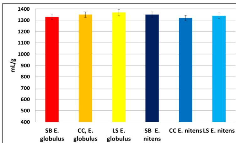
**Fig. 10.** Intrinsic viscosities of bleached pulps of *E. globulus* and *E. nitens*. The error bars present 95% confidence interval of the mean value.
