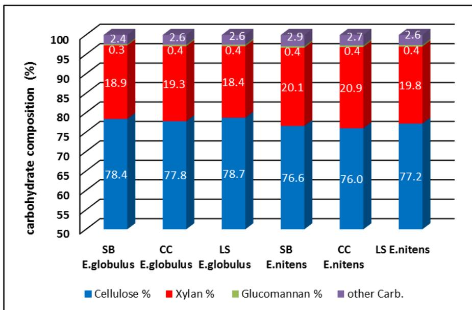
**Fig. 6.** Carbohydrate composition of brownstocks at kappa  $17 \pm 0.5$  for *E. globulus* and *E. nitens* for the three different cooking methods.
