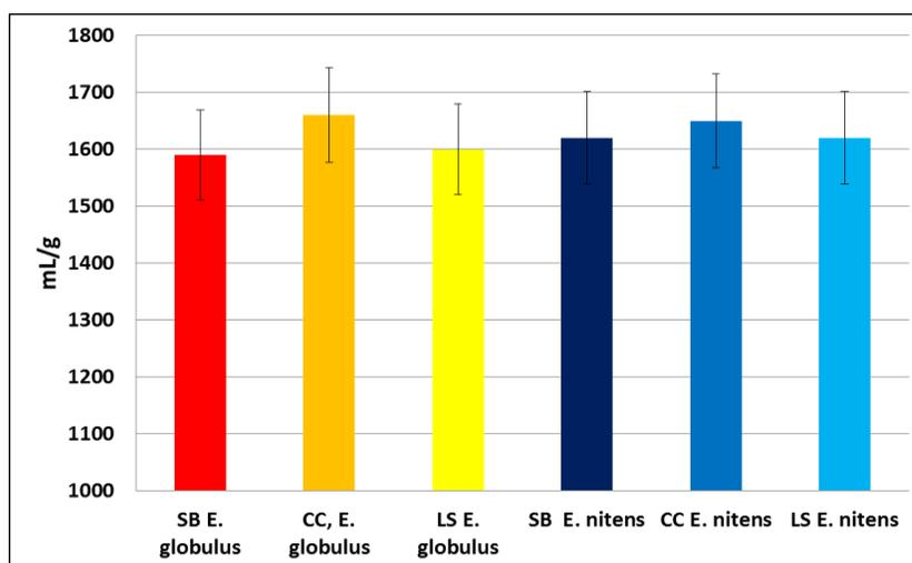
**Fig. 1.** Intrinsic viscosity of brownstocks at kappa  $17 \pm 0.5$ . The error bars present 95% confidence interval of the mean value.
