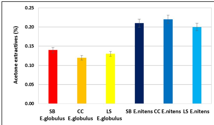
**Fig. 2.** Acetone extractives in brownstock at kappa  $17 \pm 0.5$ . The error bars present 95% confidence interval of the mean value.
