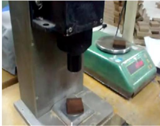
**Fig. 1.** The measurement of dimensions and weight at the IB600 laboratory testing machine
