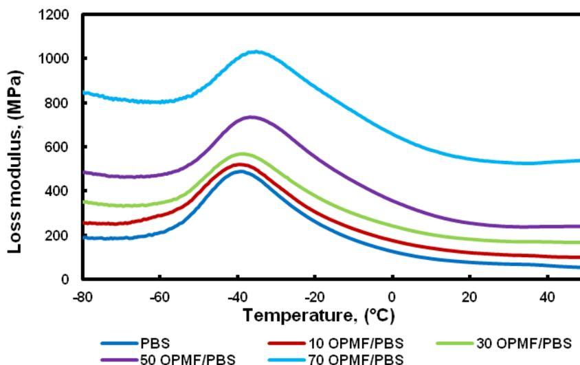
Fig. 4. Loss modulus of neat PBS and its biocomposites of various OPMF content
