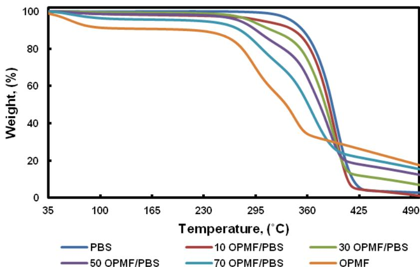
Fig. 8. TG thermograms of OPMF, PBS, and their biocomposites of various OPMF content
