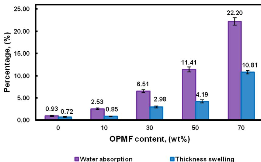
**Fig. 10.** Water absorption and thickness swelling of neat PBS and its biocomposites of various OPMF content
