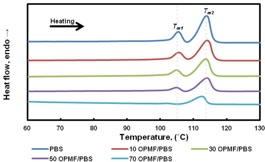
Fig. 6. DSC heating thermograms of neat PBS and its biocomposites of various OPMF content
