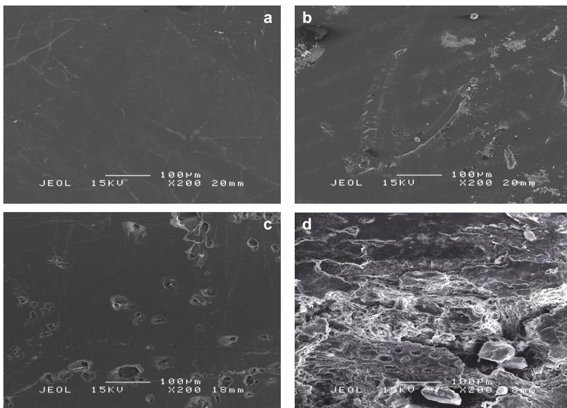
**Fig. 12.** Scanning electron micrographs of neat PBS (a and b) and biocomposites at 70 wt% OPMF (c and d) before (left) and after (right) soil burial test
