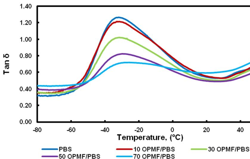
Fig. 5. Loss factor of neat PBS and its biocomposites of various OPMF content
