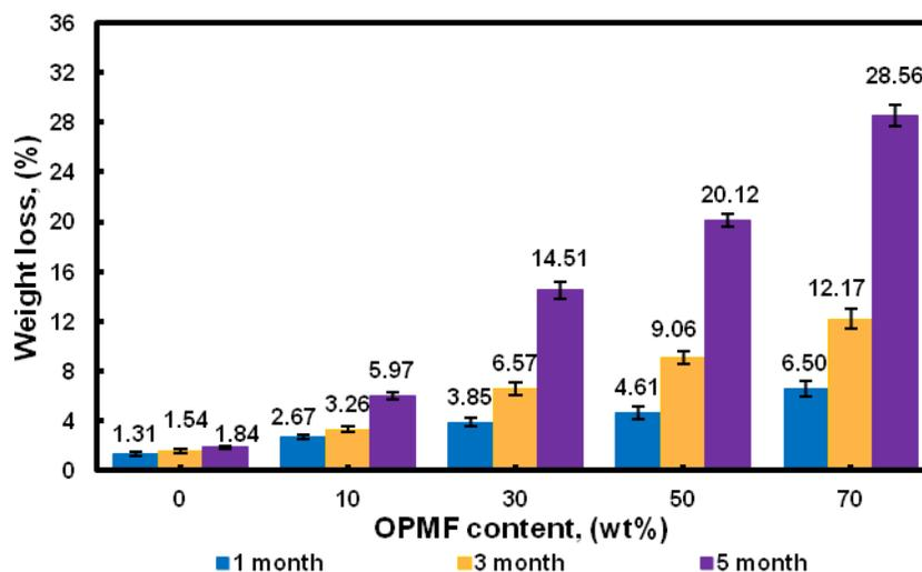
**Fig. 11.** Weight loss of PBS and its biocomposites of various OPMF content under natural soil buried test
