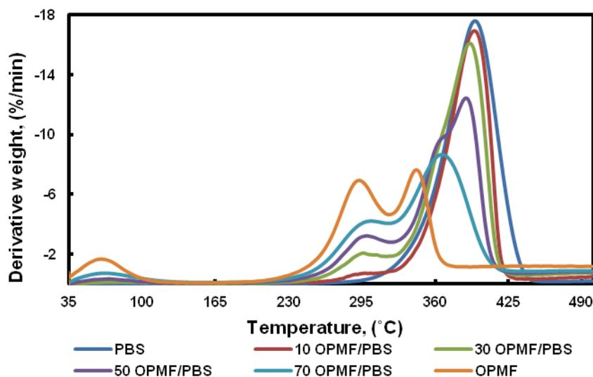
**Fig. 9.** DTG thermograms of OPMF, PBS, and their biocomposites of various OPMF content
