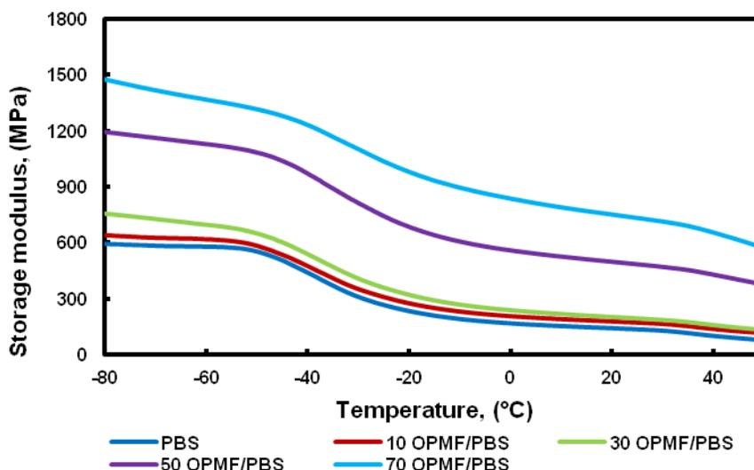
**Fig. 3.** Storage modulus of neat PBS and biocomposites of various OPMF content
