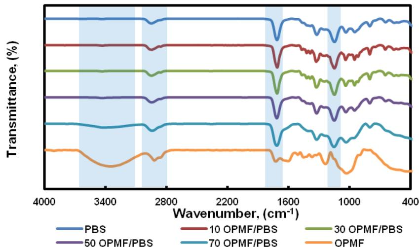
**Fig. 2.** FTIR spectra of neat PBS, OPMF, and biocomposites of various OPMF content
