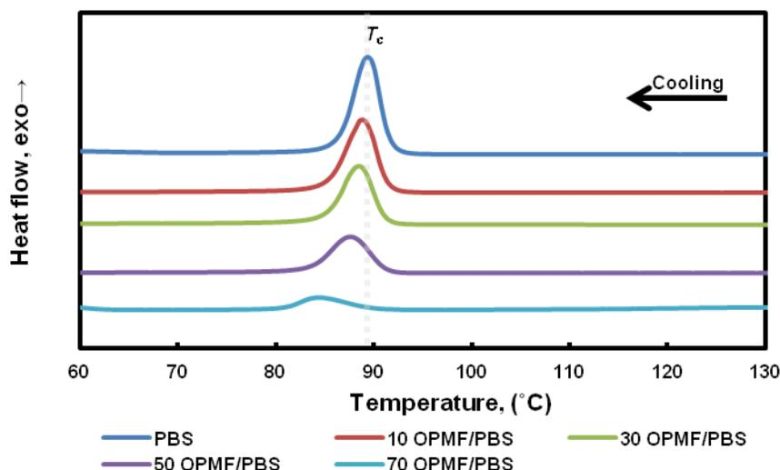
**Fig. 7.** DSC cooling thermograms of neat PBS and its biocomposites of various OPMF content
