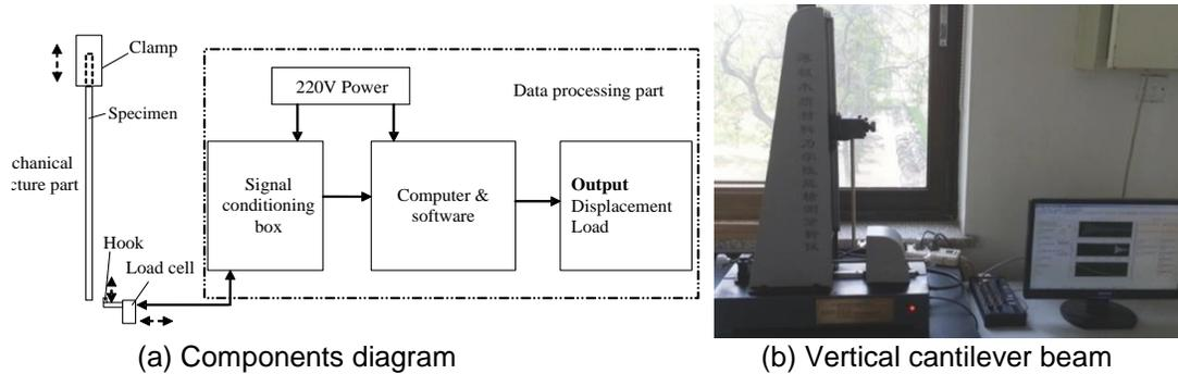
Fig. 2. Cantilever beam test apparatus
