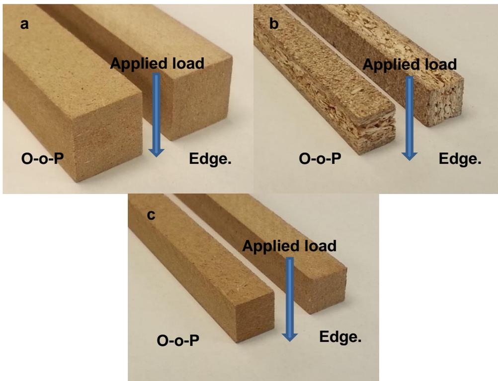
Fig. 3. Square beams tested: (a) 20 mm thick MDF; (b) 12 mm thick PB; and (c) 12 mm thick MDF. The top surfaces as seen in the beam on the left in each group had similar surfaces as those of the larger panel. The applied loading was out-of-plane (O-o-P) to the panel surfaces. The top panel surfaces were rotated 90° for beams on the right in each group. The applied loading was edgewise (Edge.) to the panel surfaces. Note: It is easier to see orientation differences for the beams in (b).
