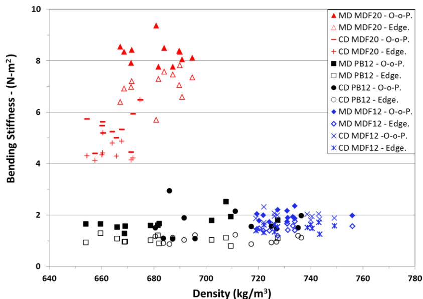
**Fig. 4.** Bending stiffness for the square cut beams from large sheets of material along the longitudinal (MD) direction and cross-wise (CD) direction of the panel. The panels include 20 mm thick MDF, 12 mm thick PB, and 12 mm thick MDF. Each beam was oriented with the surfaces of the beam out-of-plane and edgewise with the loading direction.
