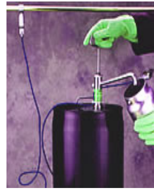
Dispensing pump with Bonding and grounding wires and alligator clips.
