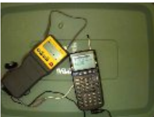
TI-83 calculator with CBL unit and pH probe. Image provided by author Lisa L. Grable.
