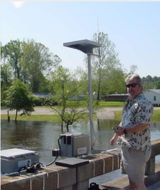
Sensors set up by Ted Dodson on a bridge over the Neuse River continually sample water quality as part of the RiverNet system. ●
