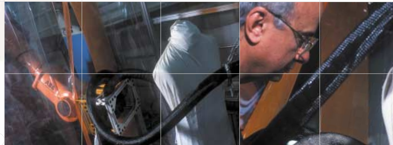
Robotic Fiber Assembly and Control system can mold a non-woven fabric of meltblown nanofibers to a mannequin, manufacturing a garment without cutting or sewing •
