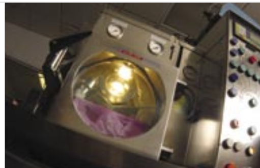
A small dyeing machine in the College of Textiles helps test HueMetrix's "right first time" system. ●
