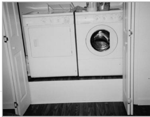
Front-loading washer and dryer with front mounted controls raised on a platform to minimize bending and stooping and place items inside the appliances within easier reach.
