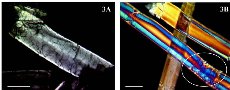
**Fig. 3A and B.** Appearance of unbleached kraft pulp fibres in polarized light after degradation by Celluclast (endoglucanase + cellobiohydrolase). **Fig. 3A:** Mill 4 earlywood fibre and **Fig. 3B:** Lab 4 latewood fibres. Bars are 35 and 30  $\mu\text{m}$  respectively. A large dislocation is seen in the latewood fibre in the ellipse.
