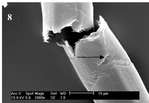
**Fig. 7.** Early phase of cellulase (0.3 ml Celluclast) action producing numerous clefts/ grooves in the outer fibre wall (see black arrows). An artefact crack is shown at the line to the left.
