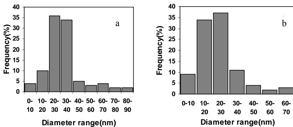
**Fig. 3.** Size distributions for the diameters of a) the homogenized unbleached pulp, and b) the homogenized bleached pulp
