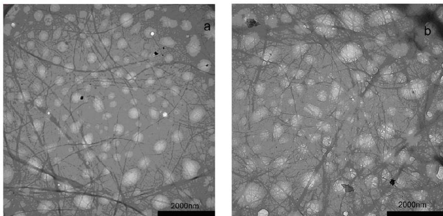
**Fig. 2.** Transmission electron micrographs of kenaf nanofibers after 40 pass through the high-pressure homogenizer: a) Unbleached nanofiber; b) bleached nanofiber (scale bar: 2000 nm).
