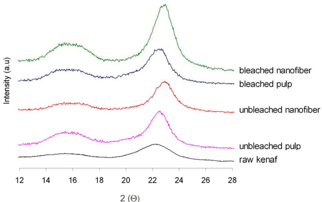
**Fig. 5.** X-ray diffraction patterns of the raw kenaf, unbleached pulp, bleached pulp, unbleached nanofibers, and bleached nanofibers.
