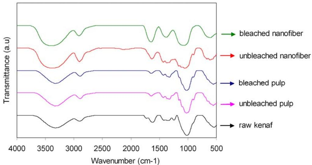
**Fig. 4.** Infrared spectra of the raw kenaf, unbleached pulp, bleached pulp, unbleached nanofibers and bleached nanofibers
