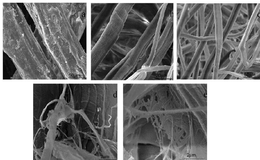
**Fig. 1.** ESEM micrographs of the structure of the kenaf fibers before and after chemical treatment for: a) raw kenaf fibers, b) unbleached pulp, c) bleached pulp, d) fibers after cryo-crushing and treatment in a PFI mill, and e) bleached pulp after cryo-crushing and treatment in a PFI mill
