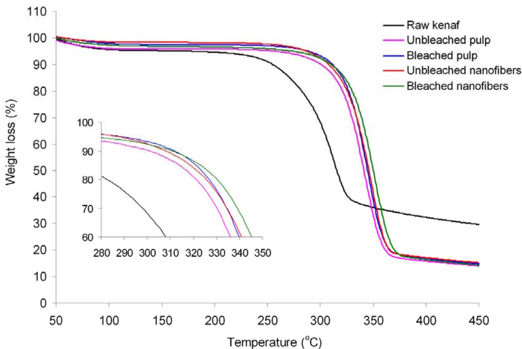
**Fig. 6.** TGA curves of raw kenaf, unbleached pulp, bleached pulp, unbleached nanofibers, and bleached nanofibers. The analysis was performed under a nitrogen atmosphere.
