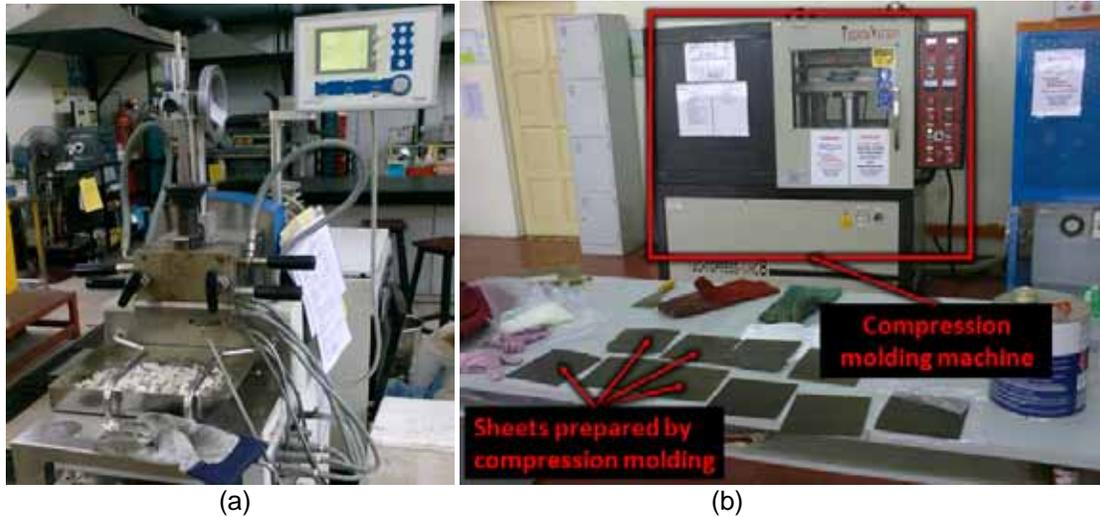
**Fig. 3.** (a) Internal mixer, (b) Compression molding machine
