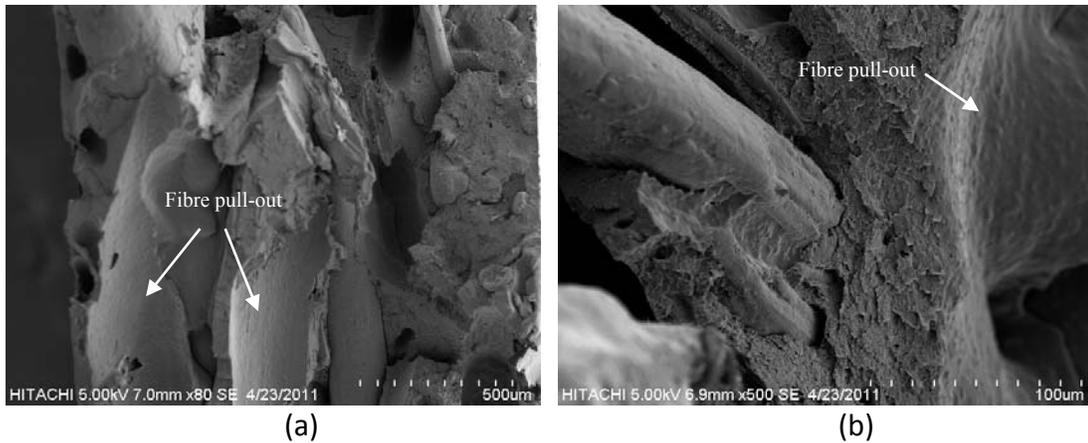
**Fig. 5.** The fracture surface of a SPF-HIPS composite with (a) the addition of 2%MAH, (b) the addition of 3% MAH
