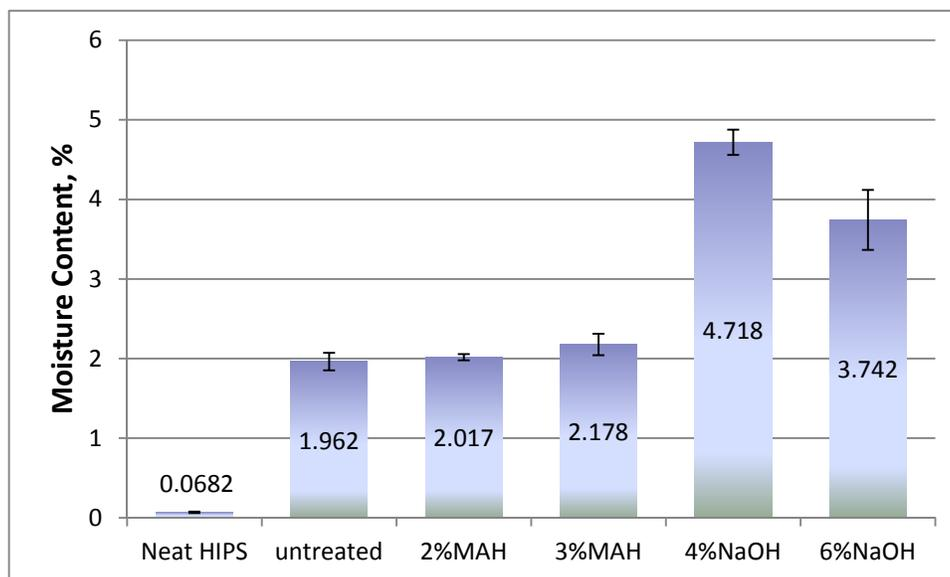
Fig. 7. The water absorption behavior of the SPF-HIPS composites, after 24 hours immersion
