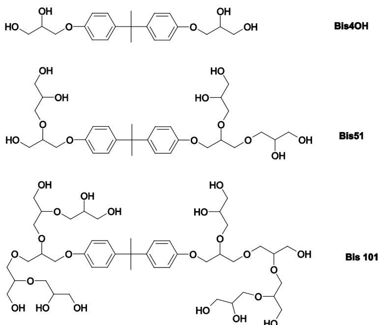
**Fig. 1.** Theoretical structures of the hyperbranched polyglycerols with bisphenol A in the core of the molecule
