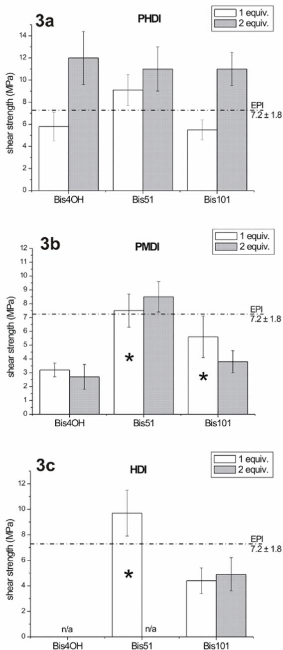
**Fig. 3.** Shear strengths of the adhesives cured with PHDI (3a), PMDI (3b) and HDI (3c). Asterisks denote unreacted NCO groups found in the cured adhesive
