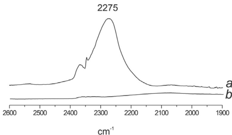
**Fig. 4.** Representative FTIR spectra of the NCO region of the cured adhesives: **a** – NCO band at  $2275\text{ cm}^{-1}$ , **b** – NCO-free spectrum
