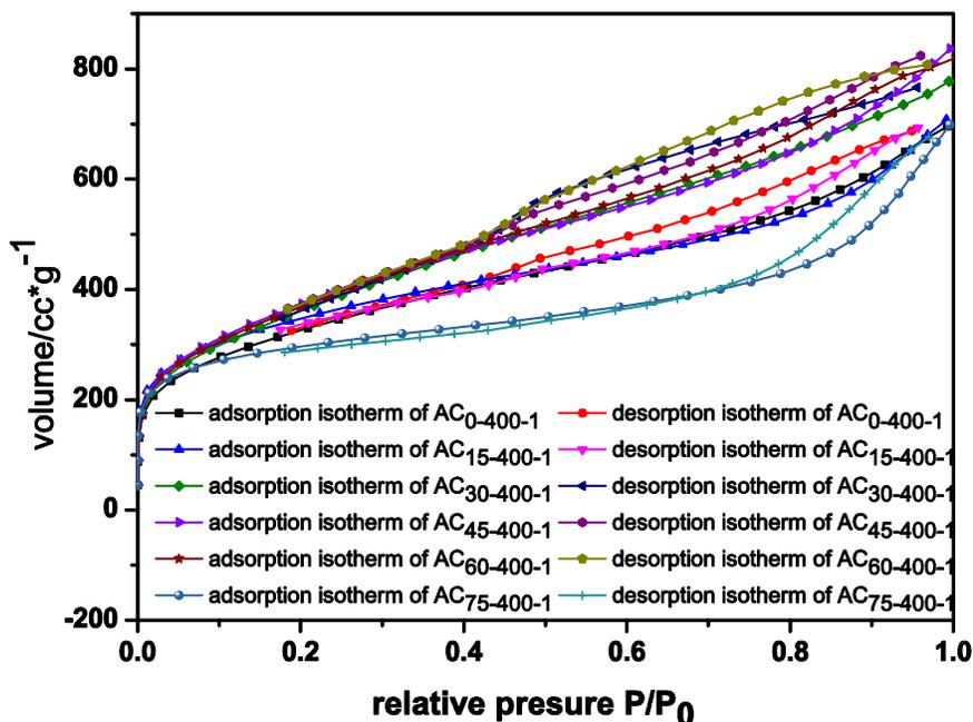
Fig. 1. Adsorption-desorption isotherm of N<sub>2</sub> at 77K
