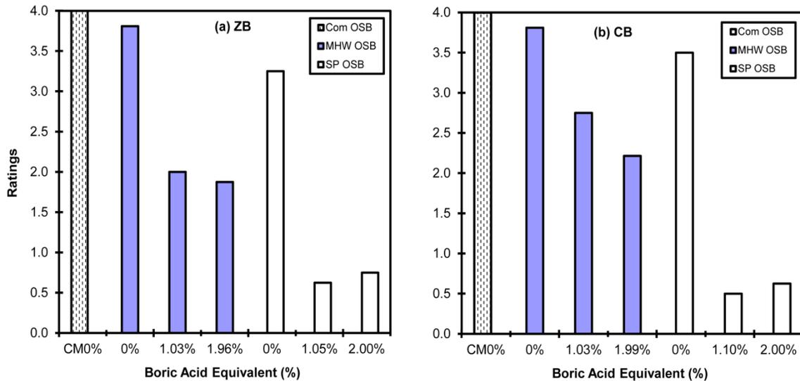
**Fig. 3.** A comparison of visual ratings of (a) ZB- and (b) CB-treated OSB exposed to mold fungi for 6 weeks
