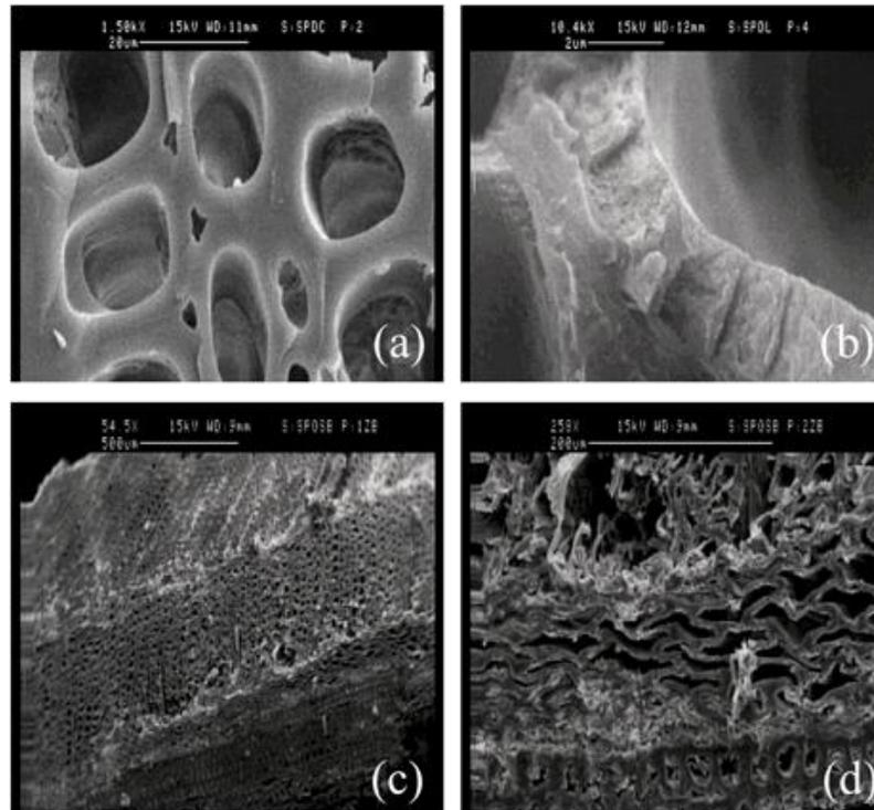
**Fig. 1.** Scanning electron micrographs of SYP wood and OSB samples unexposed and exposed to the fungi *G. trabeum*. Typical views of undecayed (a) and decayed (b) SYP tracheid cells; and typical views of undecayed (c) and decayed (d) SYP OSB.
