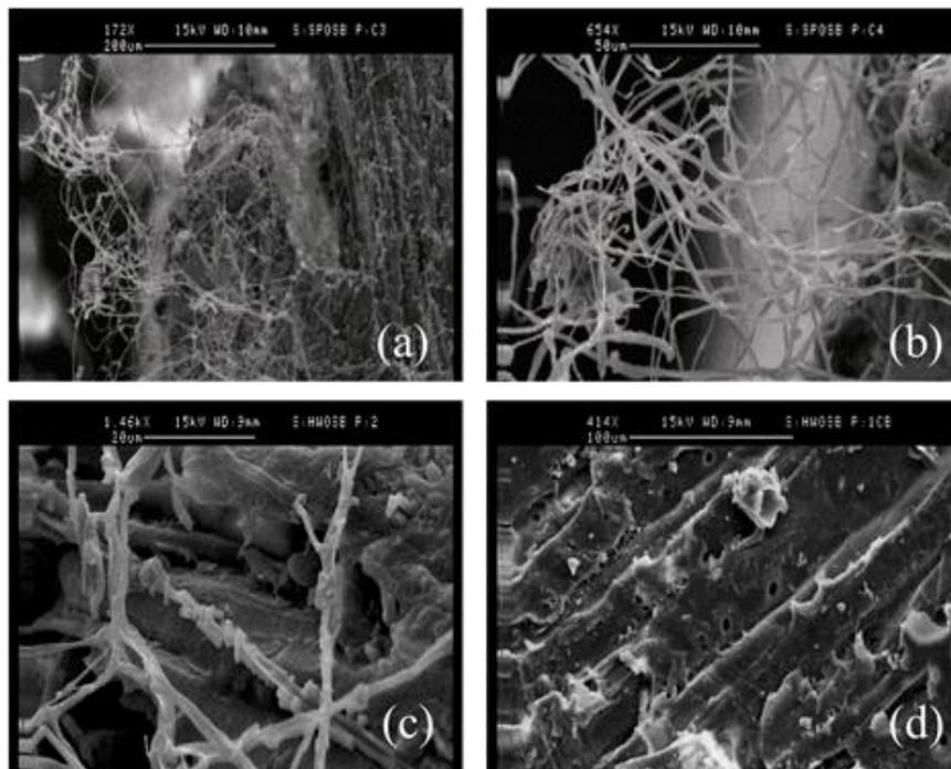
**Fig. 2.** Scanning electron micrographs of MHW and SYP OSB exposed to the fungi *G. trabeum*. (a) and (b) hyphal growth on tracheid cell of untreated SYP OSB, (c) hyphal growth on untreated MHW OSB, (d) no hyphal growth on CB-treated MHW OSB (1.0% BAE).
