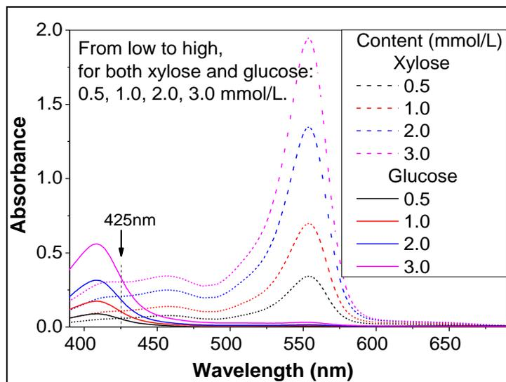
**Fig. 2.** Spectra of derivatives from various concentrations of xylose and glucose. Note: 425 nm is the isosbestic wavelength.
