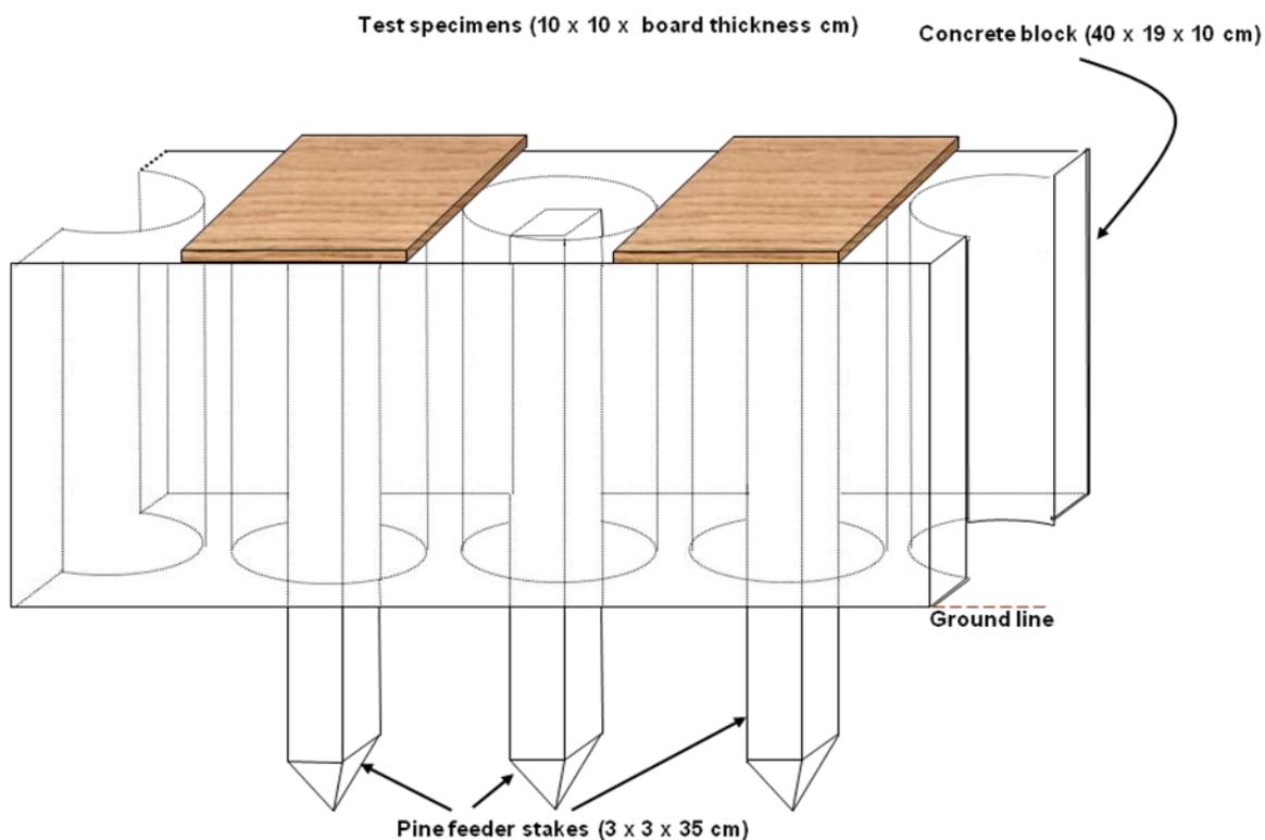
**Fig. 1.** Installation details of specimens and feeder stakes
