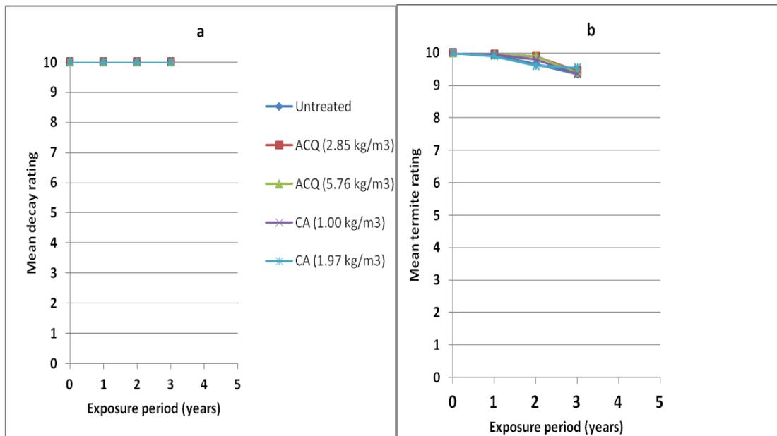
**Fig. 4.** Progress in decay (a) and termite attack (b) on untreated, ACQ-treated, and CA-treated MDF during 36 months of field exposure
