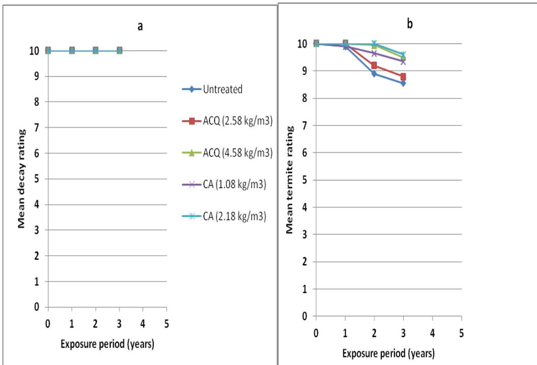
**Fig. 6.** Progress in decay (a) and termite attack (b) on untreated, ACQ-treated, and CA-treated PB during 36 months of field exposure
