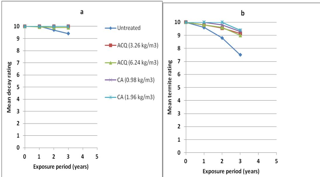
**Fig. 2.** Progress in decay (a) and termite attack (b) on untreated, ACQ-treated, and CA-treated SWP during 36 months of field exposure
