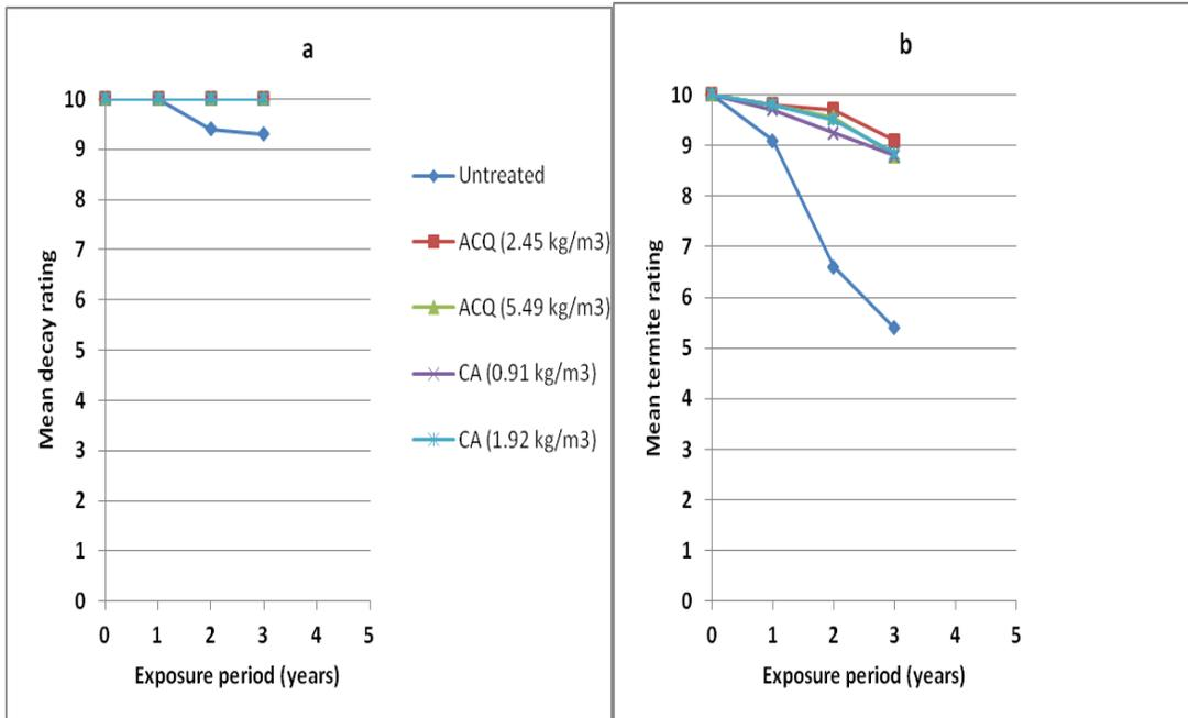
**Fig. 5.** Progress in decay (a) and termite attack (b) on untreated, ACQ-treated, and CA-treated OSB during 36 months of field exposure
