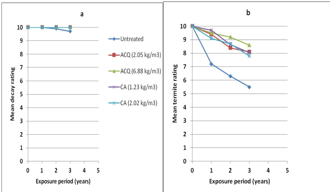
**Fig. 3.** Progress in decay (a) and termite attack (b) on untreated, ACQ-treated, and CA-treated HWP during 36 months of field exposure
