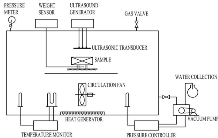
Fig. 1. Schematic of the experimental set-up of the ultrasound-vacuum dryer
