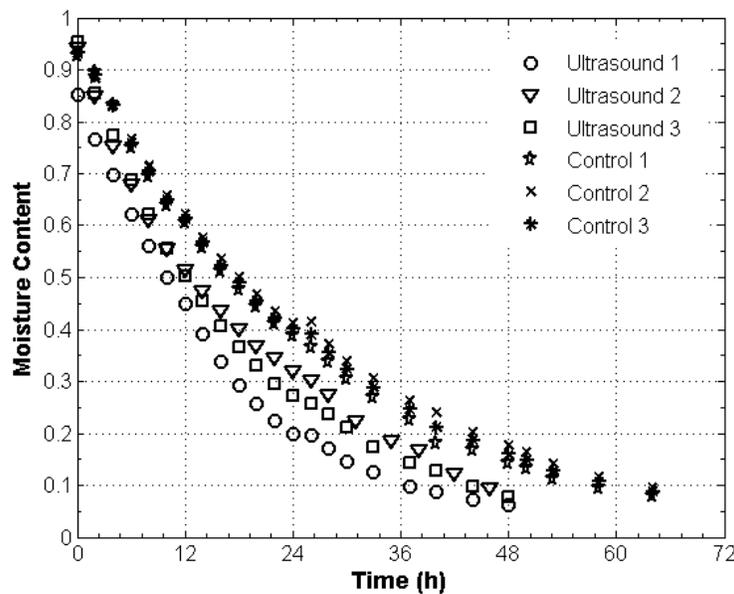
**Fig. 3.** Comparable drying kinetics of Chinese walnut specimens vacuum dried with and without ultrasonic assistance at 0.08 MPa pressure and 60°C
