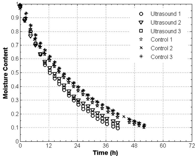
**Fig. 2.** Comparable drying kinetics of Chinese walnut specimens vacuum dried with and without ultrasonic assistance at 0.05 MPa pressure and 60°C
