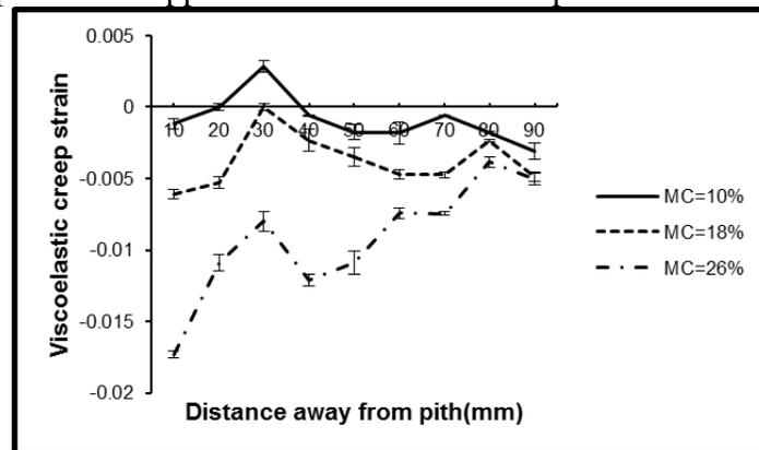
**Fig. 6.** The radial distribution of viscoelastic creep strain at different MCs
