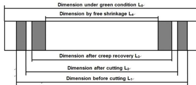
**Fig. 3.** The size of the strain slice at different drying states
