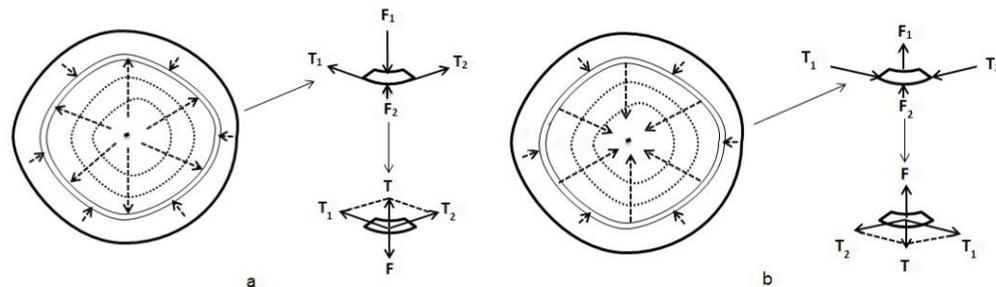
Fig. 4. Diagram of stress analysis in wood disks
