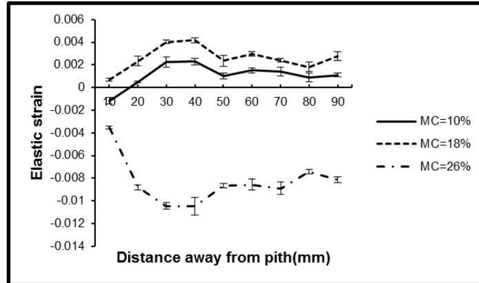
**Fig. 5.** The radial distribution of elastic strain at different MCs
