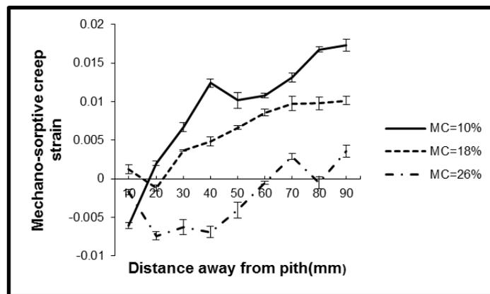
Fig. 7. The radial distribution of MS creep strain at different MCs
