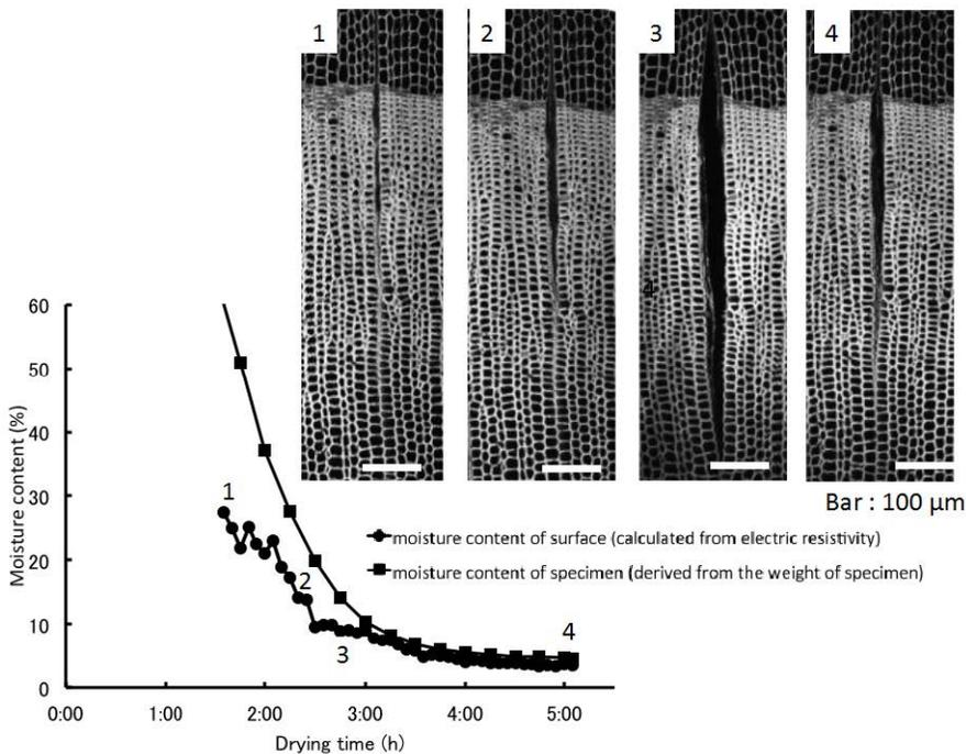
**Fig. 6.** Relationship between moisture content and microcrack generation in *Cryptomeria japonica* red heartwood (upper) and black heartwood (lower); two types of moisture content, one calculated from electrical resistivity and one determined from the weight of the specimen, are shown.
