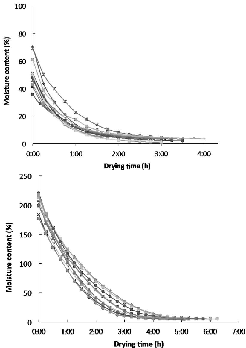
**Fig. 4.** Relationship between drying time and moisture content as determined from the weights of *Cryptomeria japonica* specimens (upper: 12 samples of red heartwood, lower: 10 samples of black heartwood).
