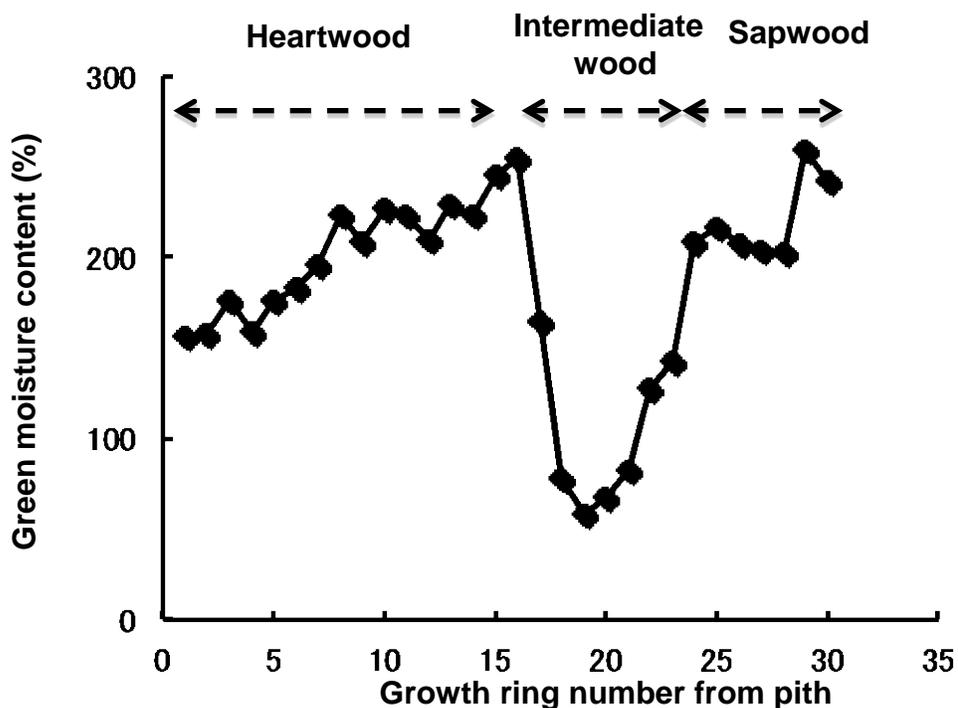
**Fig. 2.** Green moisture content of *Cryptomeria japonica* black heartwood from pith to bark; the moisture contents of heartwood and sapwood were high in comparison to that of intermediate wood.
