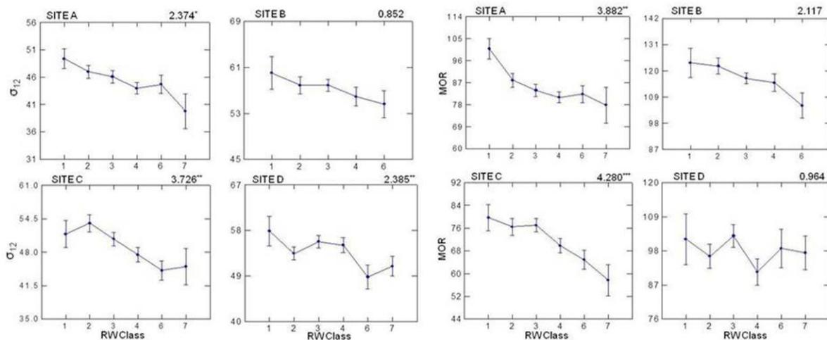
**Fig. 2.** ANOVA analysis of the effect of ring width (RW) class on compressive strength and MOR. The numbers above the graphs are F values with significant probability: \*  $p < 0.05$ , \*\*  $p < 0.01$ , \*\*\*  $p < 0.001$ .
