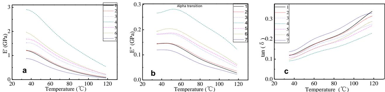
**Fig. 3.** Plots of (a)  $E'$ , (b)  $E''$ , and (c)  $\tan \delta$  versus temperature for the HDPE and BPF/HDPE and BF/HDPE composites
