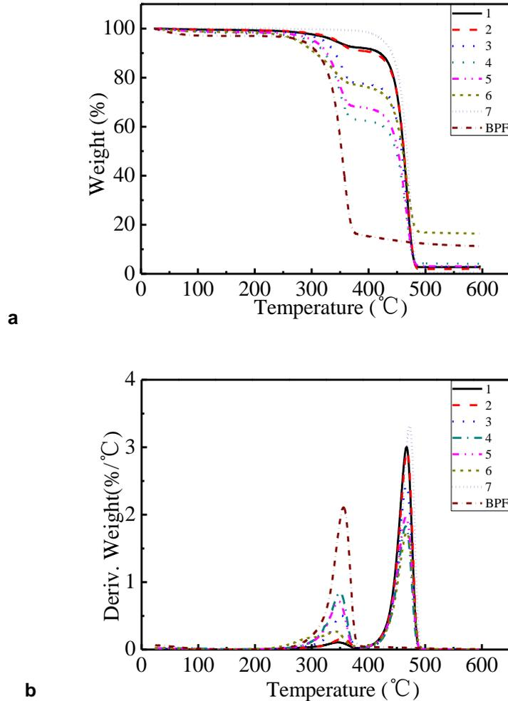
**Fig. 2.** The (a) TGA curves and (b) DTA curves of BPF, HDPE, BPF/HDPE composites, and BP/HDPE composites
