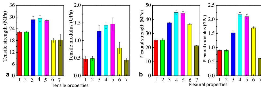
**Fig. 1.** Mechanical properties of HDPE and BPF/HDPE and BF/HDPE composites: (a) tensile properties and (b) flexural properties
