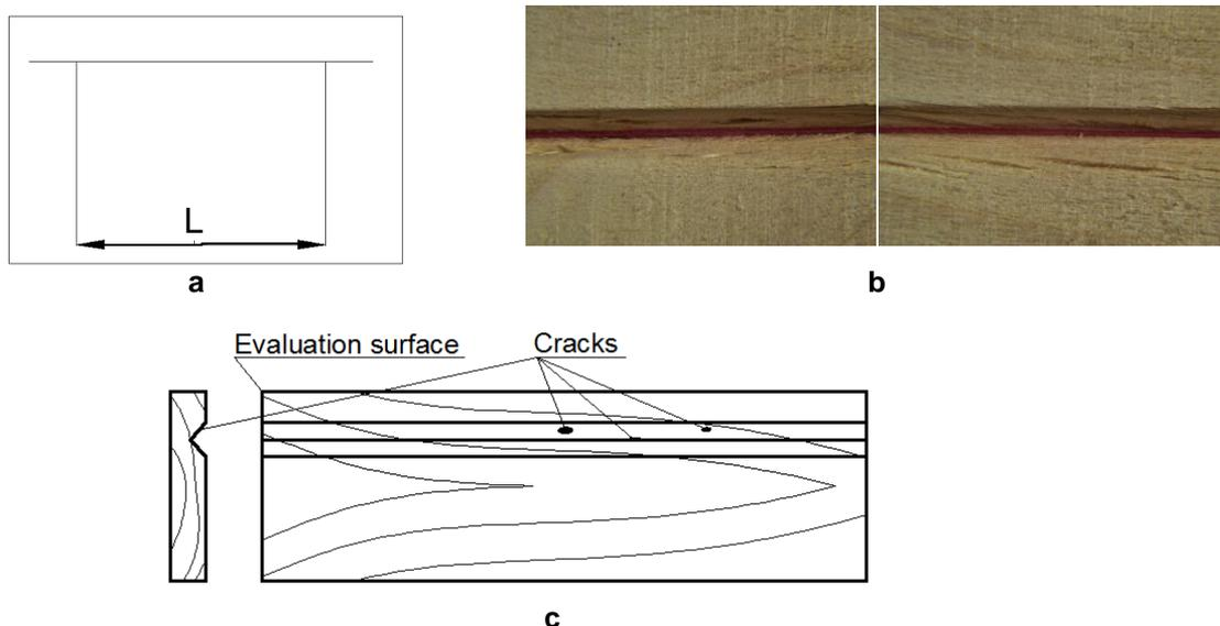
**Fig. 7.** Use of SURFACE software. (a) Schematic illustration of calibration image, (b) digital images used to calculate the area of the crack, and (c) measurement and evaluation principle of SURFACE software
