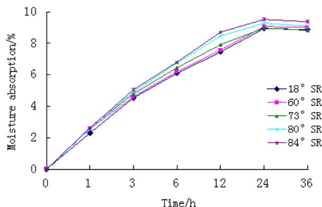
**Fig. 2.** Effects of the beating degree of micronized fibers on moisture absorption
