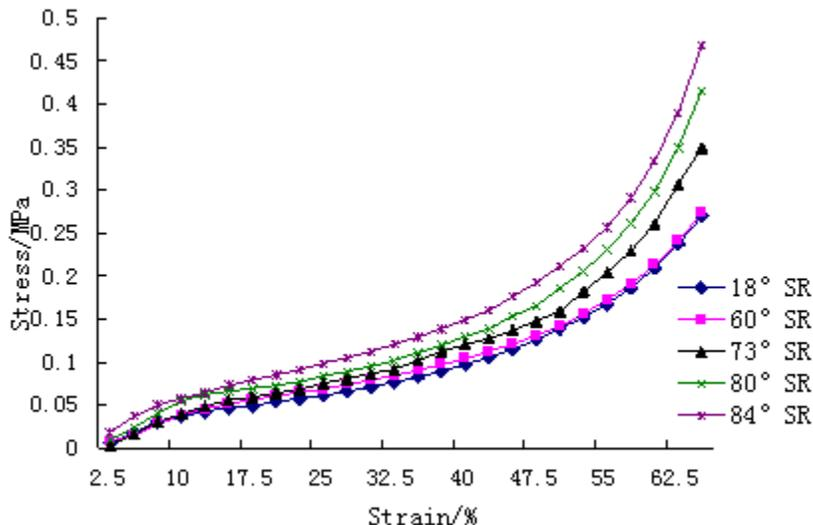
**Fig. 3.** Stress-strain curves of the samples prepared with micronized fibers of different beating degrees
