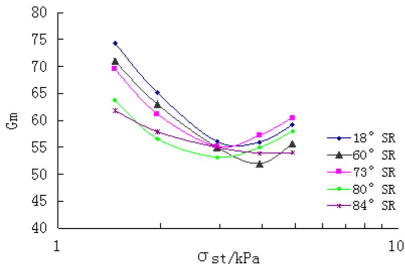
**Fig. 4.** The  $G_m-\sigma_{st}$  curves of foam buffer materials prepared with micronized fibers of different beating degrees
