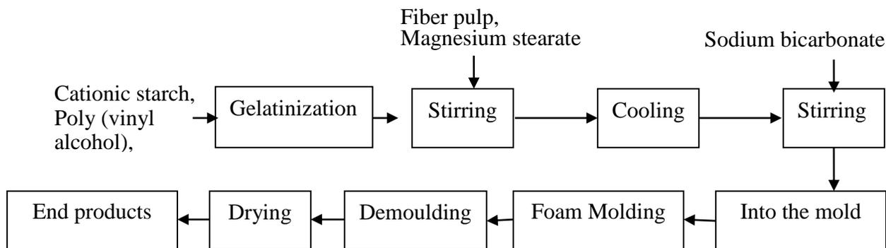
**Fig. 1.** The flow chart of the preparation of foam buffer materials
